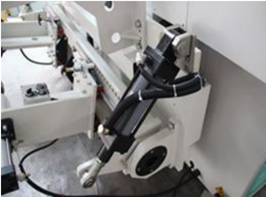
Unwinding Hydraulic Lifting
